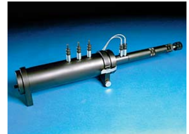
Impedance Tube Apparatus (per ASTM E-1050)
