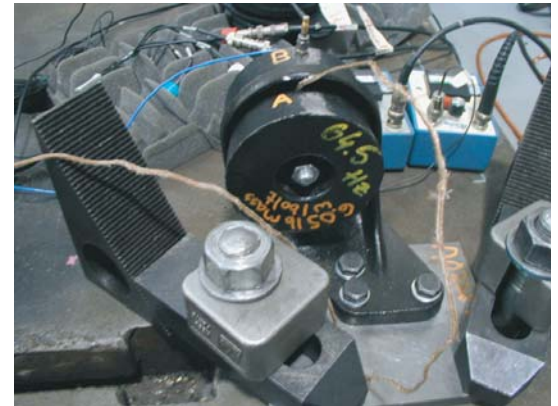
Impact test while mounted to bed plate
