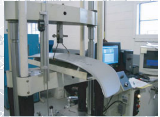
Testing the Strength of a Spoiler Using the 60,000 lb. Tinius Olsen Machine
