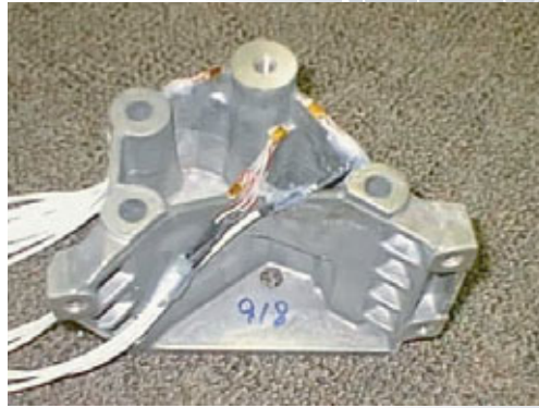
Custom Strain Gauging of a Critical Part
