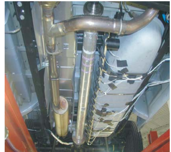
Propshaft Acoustic Mode Measurement
