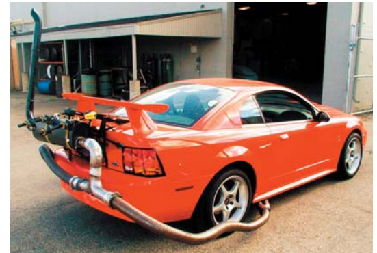
Second Muffler to Reduce Exhaust Noise for Intake Testing
