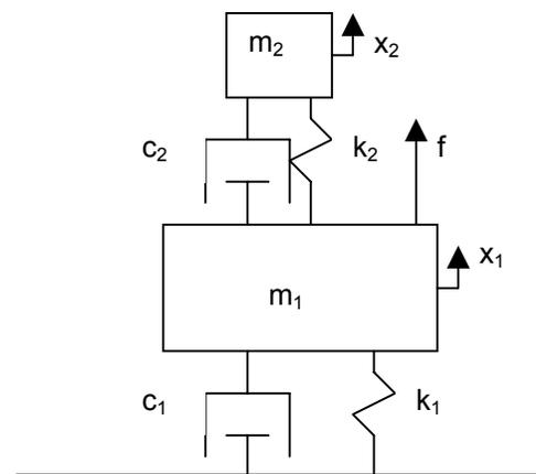
Figure 1 – Model of Base Structure with Damper.
