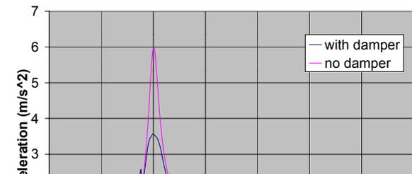
Figure 11 – Effectiveness of 95% Iron Powder Filled Particle Damper with Structural Excitation of 60N.
