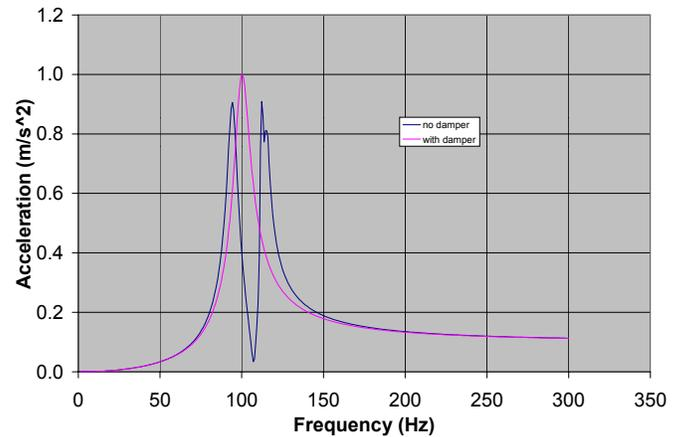
Figure 4 – Effectiveness of 95% Lead Filled Particle Damper with Structural Excitation of 10 N.
