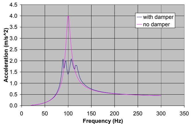
Figure 10 – Effectiveness of 95% Iron Powder Filled Particle Damper with Structural Excitation of 40N.
