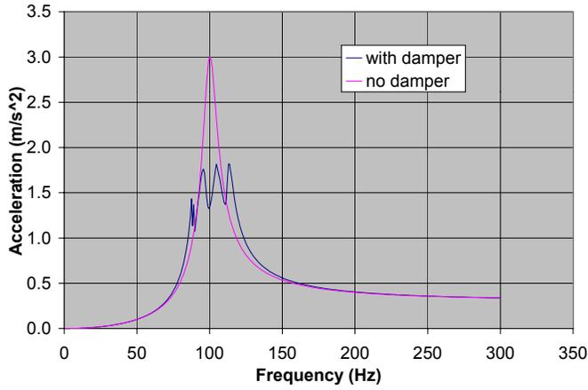
Figure 6 – Effectiveness of 95% Lead Filled Particle Damper with Structural Excitation of 30 N.
