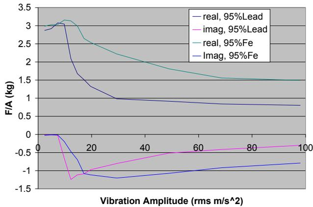
Figure 2 – Measured Real and Imaginary Masses for the Particle Dampers.
