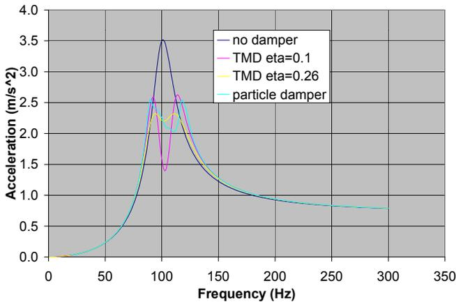
Figure 12 – Effectiveness of TMD and Iron Filled Particle Damper on a Modified Base Structure (10% Damping).
