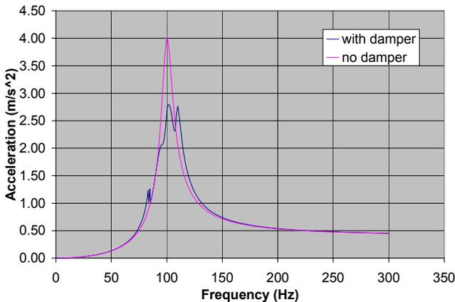
the performance does not degrade as much at higher excitation levels. The best performance (52.2%) is better than the TMD with  $\eta = 0.1$  (56.9%), but worse than the TMD with  $\eta = 0.25$  (47.5%)
