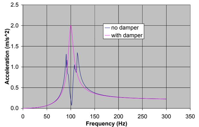
Figure 5 – Effectiveness of 95% Lead Filled Particle Damper with Structural Excitation of 20 N.
