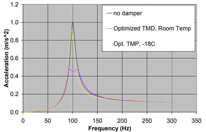
Figure 13 – Effect of Temperature on the Optimized TMD.
