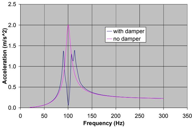
Figure 7 – Effectiveness of 95% Lead Filled Particle Damper with Structural Excitation of 40 N.
