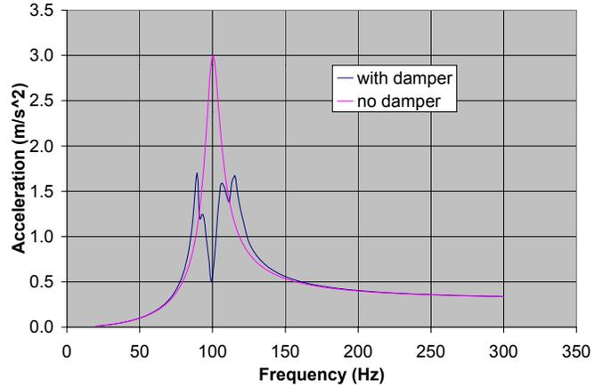
Figure 9 – Effectiveness of 95% Iron Powder Filled Particle Damper with Structural Excitation of 30N.
