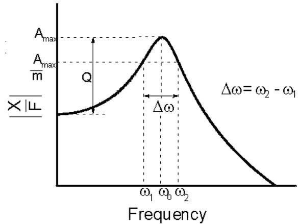
Figure 5. Compliance Transfer Function of a SDOF System
