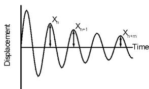
Figure 4. Transient Response of a Classically Underdamped SDOF System
