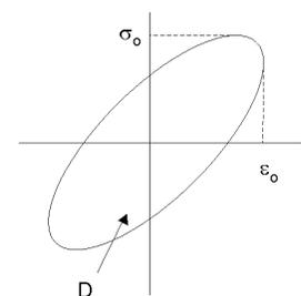
Figure 6. Typical Hysteresis Loop for a Viscoelastic Material
