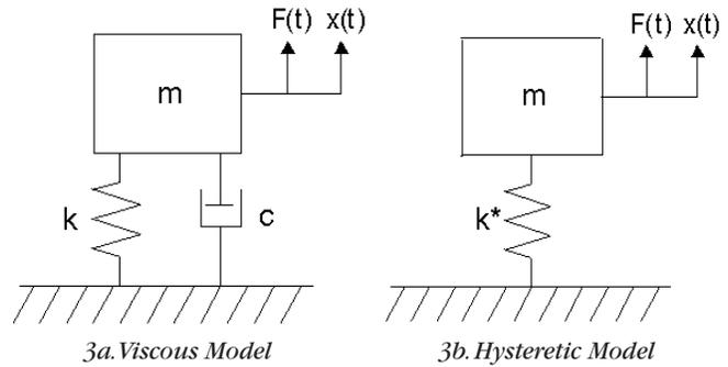
Figure 3. Single-Degree-of-Freedom Damping Models
