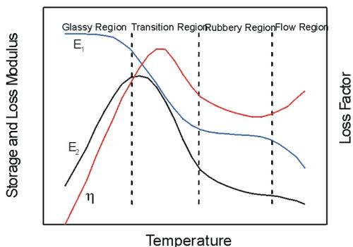
Figure 2. Variation of Complex Modulus with Temperature for a Typical Viscoelastic Material
